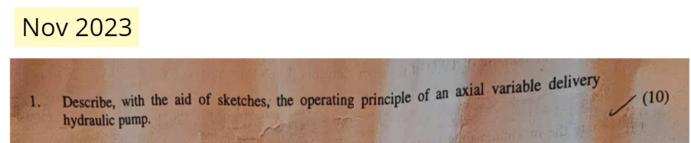
An axial variable displacement hydraulic pump uses a combination of pistons, a cylinder block, and a swash plate to convert rotational input from a drive shaft into variable fluid flow. Here's a breakdown of its operation:
